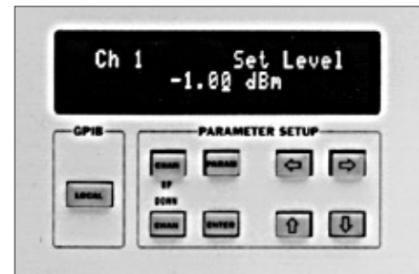
The display always shows the selected module channel in the upper left corner.
